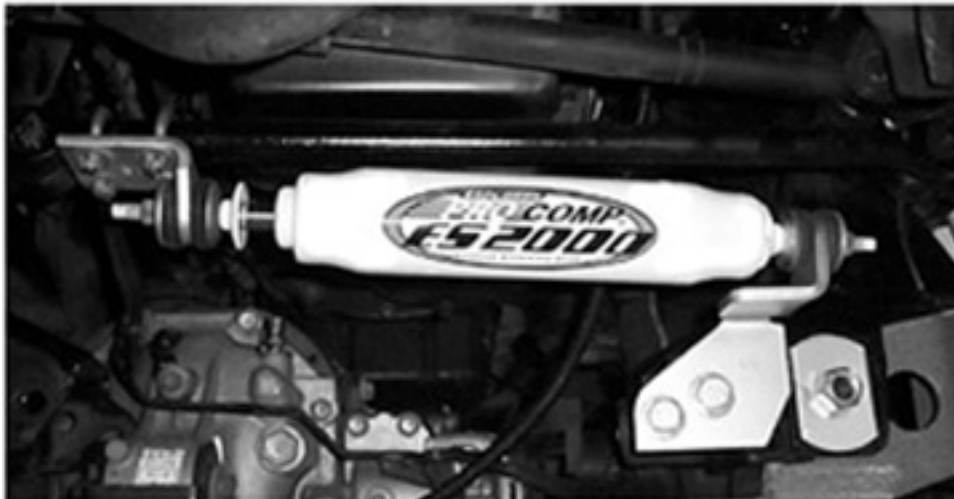
SHOWN ON VEHICLE WITH 4" SUSPENSION LIFT, ON STOCK VEHICLE LOWER BRACKETS LOCATES IN SAME LOCATION.
